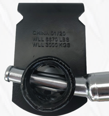
Winch Bar inserted through both end cap holes
